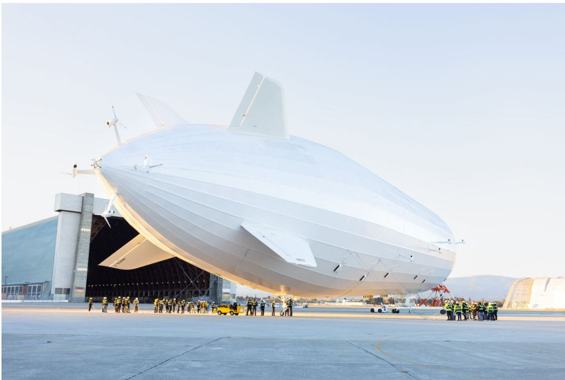
Figure 1. The P1 proof of concept airship, a flight test vehicle measuring almost 124m, took flight in 2024 for the first time. ( https://ltaresearch.com/ ) which represents the current forefront of the industry.
